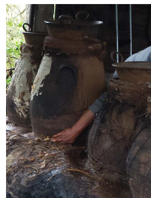
sealing the space between the pot and the condensing chamber
