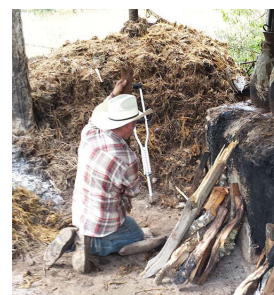
Tending the fire. Note that he's split the wood into thin pieces = more control of the heat of the fire
